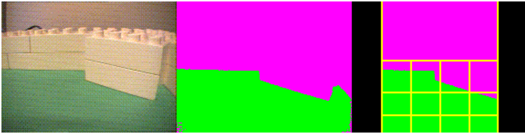
Figure 6.2: The image processing. At the left the original image. In the middle the colour segmented image. At the right the 13 regions of the visual state-space division.
