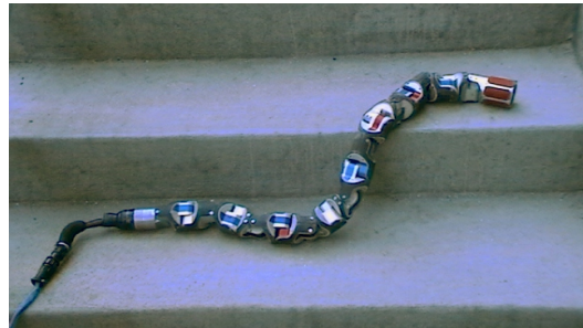
Fig. 1: A hyper-redundant snake robot, shown on an outdoor staircase.
